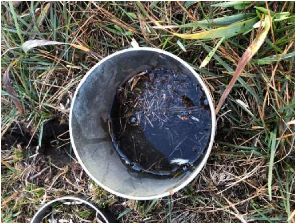
Water infiltration test on pasture, fall 2019.
